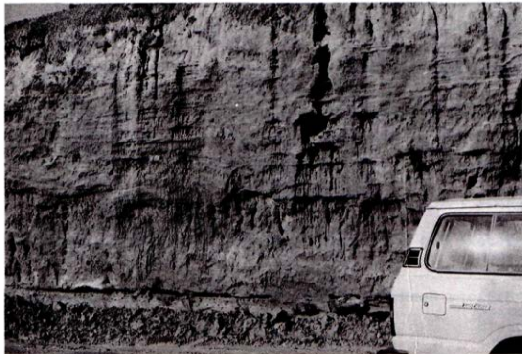
Parilla Sand - Aubrey Pit. The Shire of Warracknabeal extracts sandstone for road maintenance and construction from this public land site.
